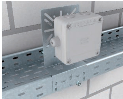
Mounting plate with quick fastening Fastening of the mounting plate, type MP, on the cable tray. The mounting plate can be fastened to the rail with quick connectors, and permanently fastened using truss-head bolts of type FRS B.
