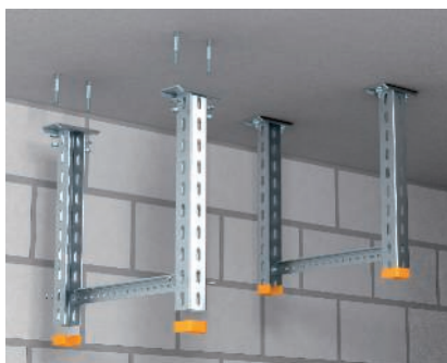
Traverse Mounting of U suspended supports US 3 K, US 5 K and US 7 K under the ceiling using bolt ties and a trapeze, consisting of U profile US 3, US 5 or US 7.
