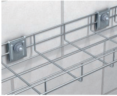
Wall mounting of mesh cable trays Wall mounting of mesh cable trays with wall bracket, type K 12 1818. Maximum mesh cable tray width 200 mm.
