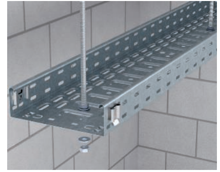
Centre suspension with threaded rod Direct centre suspension at low loads of a cable tray with threaded rod 2078/M10.
