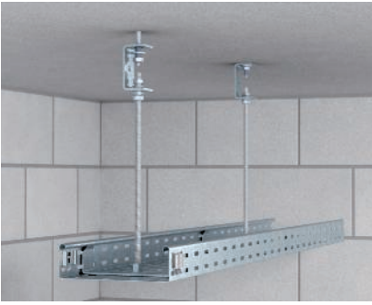
Installation of centre suspension Installation of the centre suspension MAH 60 on the ceiling using threaded rod 2078/M10 and ceiling bracket 12050. Maximum cable tray width 300 mm.
