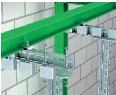
Cantilever beam with support Cantilever beams made of U support construction clamped to steel girder for installing supports.
