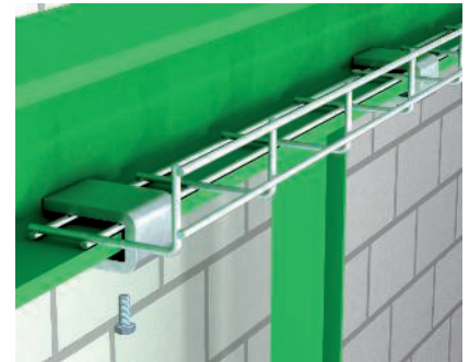
Installation of mesh angle Fastening of the mesh angle, type GW 40/80, to steel girders using beam clamps, type KL 20 or KL 30.
