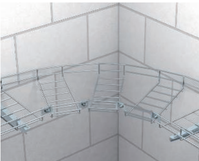
Creation of a mesh cable tray bend - round Cutting out every second grid allows the creation of mesh cable tray bends with a larger radius. Fixing takes place using corner connectors, type GEV 36.
