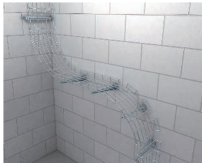
Rising and falling bends Rising and falling vertical bends can be created by cutting into every second grid of the mesh cable tray edge and bending the mesh cable tray accordingly.
