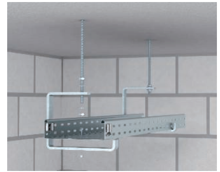
Threaded rod suspension with ceiling bracket Ceiling mounting of a cable tray with AHB ceiling bracket and threaded rod 2078/M10. Maximum cable tray width 400 mm.
